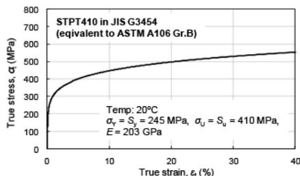
FIG. 2. — Stress-strain curve of STPT410 for FEA.
