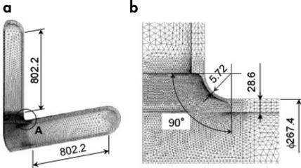
FIG. 3. — Examples of mesh division of T-joint pipes with local wall thinning. *a.* T-joint quarter model. *b.* An enlarged view of the eroded area (A)
