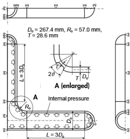
FIG. 1. — Geometry and boundary condition of the T-joint pipe.
